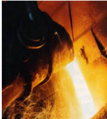
WCI Steel's Basic Oxygen Furnace where molten iron from the blast furnace is changed into liquid steel at the rate of 160,000 tons of steel a month.
